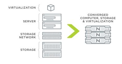
FIGURE 2: Nutanix converges compute, storage, and virtualization in simple, scalable building blocks
